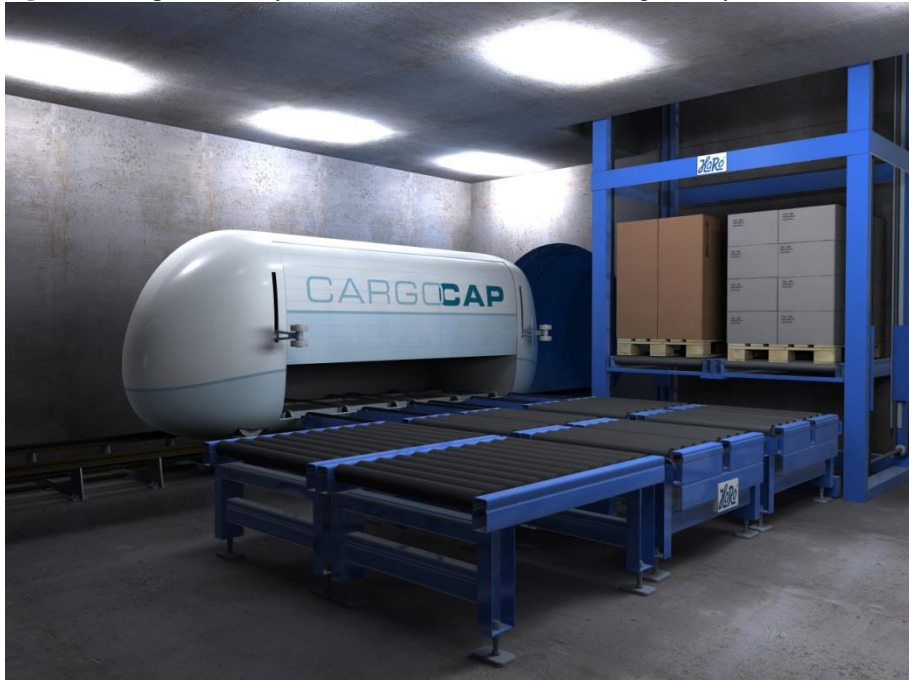
Figure 11: Caps with fully automated horizontal (un)loading conveyors
